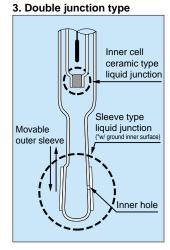
The inner filling (3.33M–KCI) tends to be less contaminated, however, for outer cell use liquid other than KCI that would not react with titration solution. For example, in silver nitrate titration for chlorine ion, use 1M–potassium nitrate instead of KCI for outer cell.
