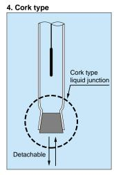
This type of electrode is used for non-aqueous titration where liquid junction is apt to generate unstable potential or when measuring samples such as paints liable to fouling liquid junction. Accordingly, the cork of the liquid junction must be periodically replaced with new one.
