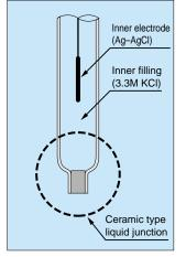
Since the inner filling flows out very little, this type of electrode is generally adequate for acid-base or redox titration of a q u e o u s s o l u t i o n . I n non-aqueous titration, potential may turn out to be unstable. Therefore, it is necessary to check on potential stability. Movable outer sleeve Unter sleeve
